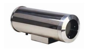
SFD Series Air-cooled Camera Housing is designed for extreme environment operation with IP68 ingress protection rating, constructed from dual layer Stainless Steel 304 or 316L materials (to be specified by client), for flowing compressed air through its interlayer for air cooling effect.
